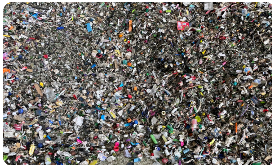
Figure 5: a selection of fines captured in the glass bunker at a materials recovery facility.
