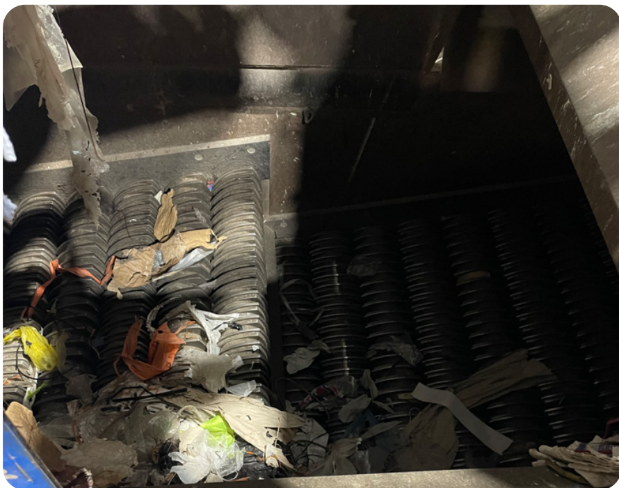
Figure 4: inside of a disc screen where materials are sorted for size, items smaller than 40 mm 2 fall between the oscillating discs.
