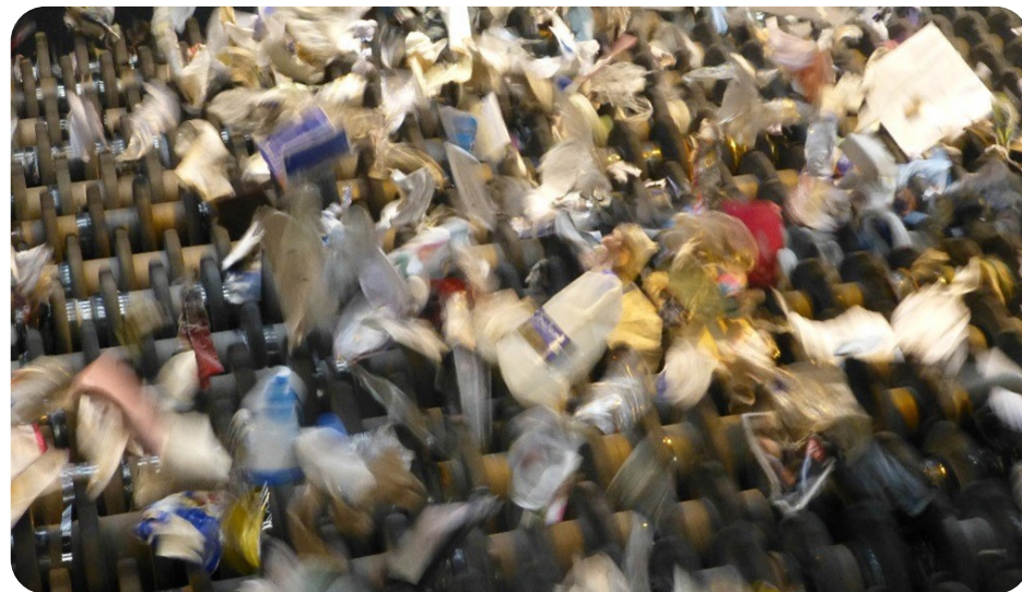
Figure 12: mixed materials being agitated on a news screen.
