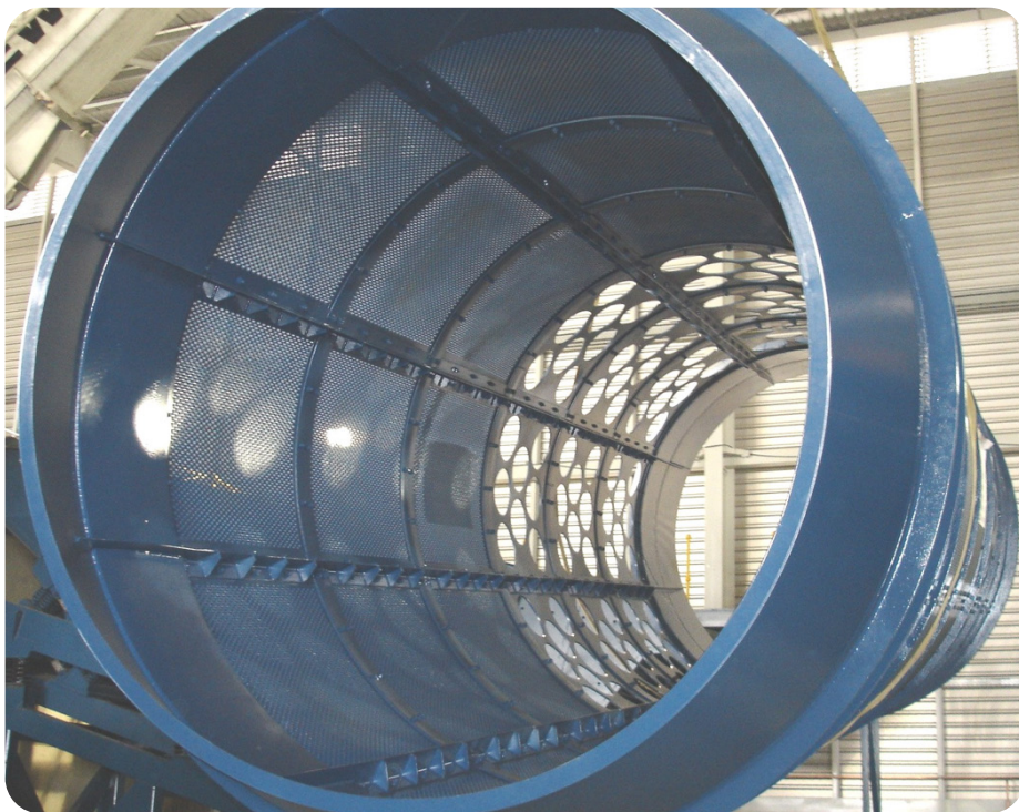
Figure 11: a trommel cylinder prior to installation.
