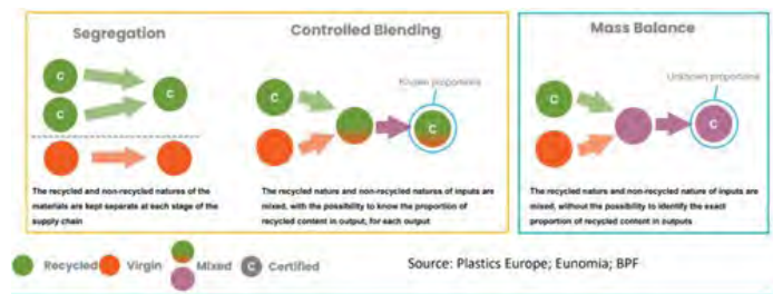
Comparison of chemical recycling processes and how mass balance can measure an otherwise unknown output 44
